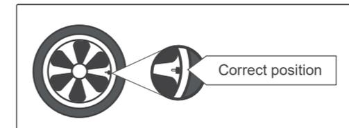
3 Place the tool to the correct position to ensure sensor activation and decode.
