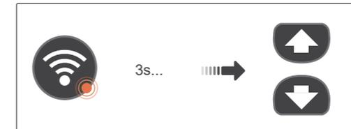
4 Press **Activate** to test the TPMS. If test passes, TPMS data will be briefly displayed for 3 seconds.
